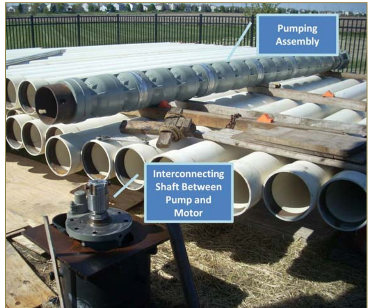
Submersible Pump and Motor Equipment
