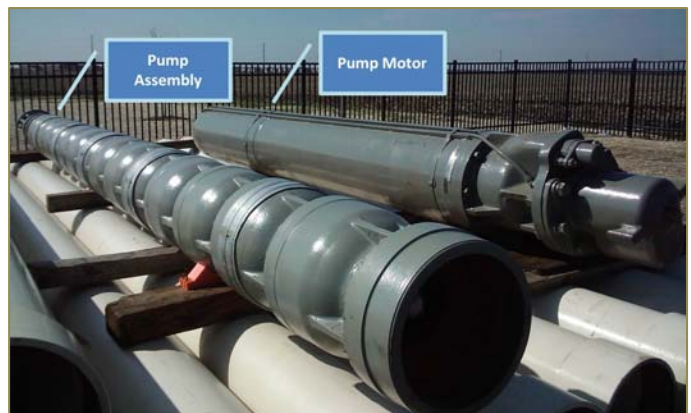
Submersible Pump and Motor Equipment
