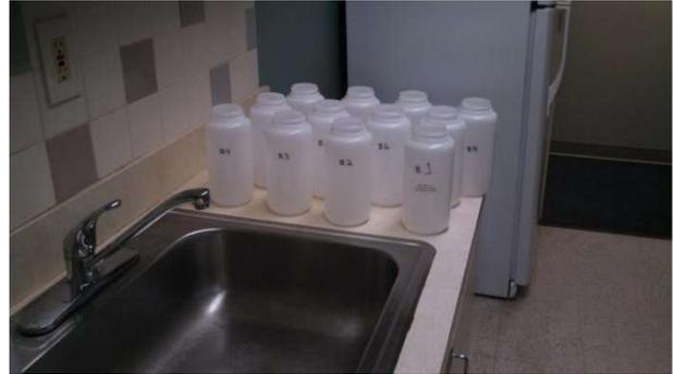
Set up sample containers before you start. The faucet must run continuously while you fill the twelve (12) containers without allowing any water to flow to drain.
