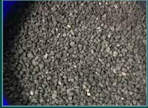
Granular Activated Carbon (GAC)
